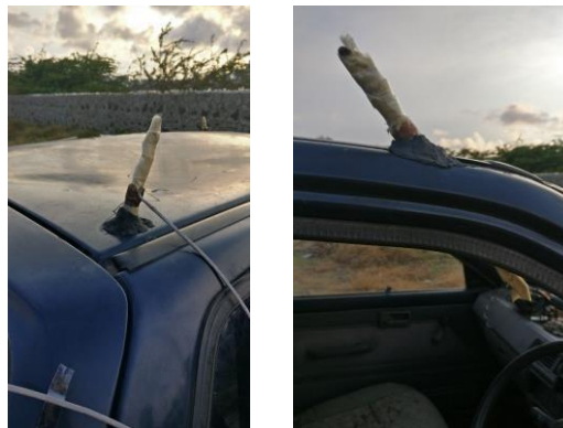
Figure 8: Installed heat pipe system
