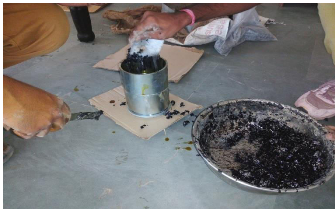
Fig 2(a): Mix prepared after mixing all the ingredient materials and the moulds in which it is to be filled
