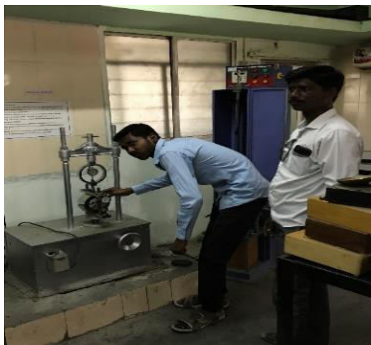
Fig 2(d): Specimen mould testing under Marshall Stability Apparatus.
