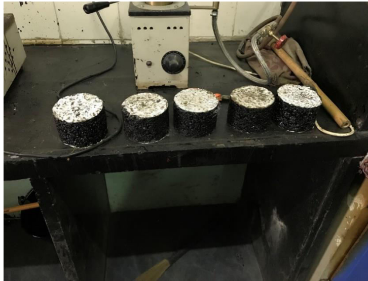
Fig 2(c): Series of specimen moulds prepared by varying P.E.T and steel slag content.
