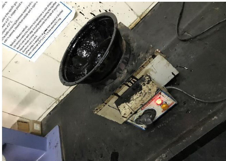
Fig 1(b): Bitumen of VG-30 grade (binder)
