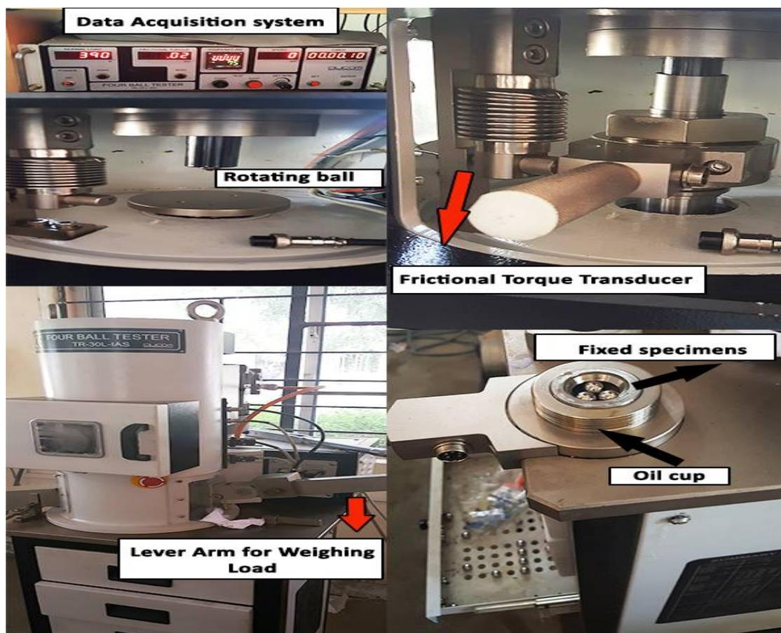
**Fig.6 : Experimental photograph of four ball tribometer**
