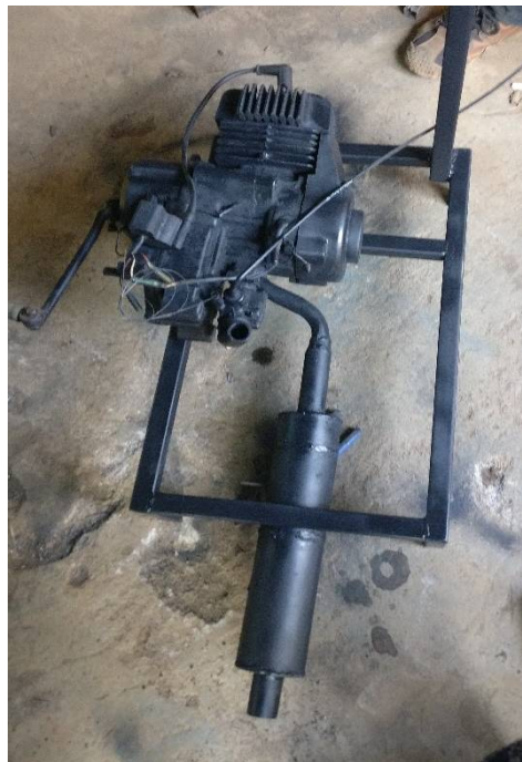
Fig 3.2: Fabricated silencer coated with limestone and charcoal
