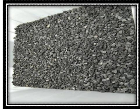
(b) COARSE AGGREGATE (Size:20mm-40mm)
