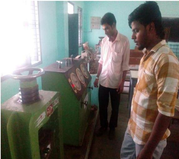
Fig 5.1(a) Compression testing machine
