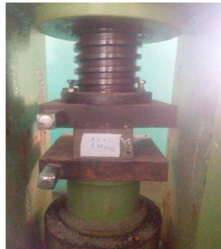
Fig 5.2(b) Testing brick in CTM
