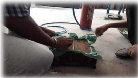
Fig 4.1(c) Filling and damping sand into mould
