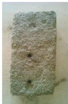
Fig5.4 Partial combination of River sand and clay brick
