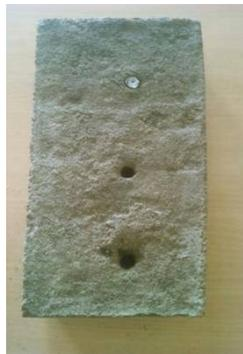
Fig 4.3 Partial combination of River sand and M-sand brick
