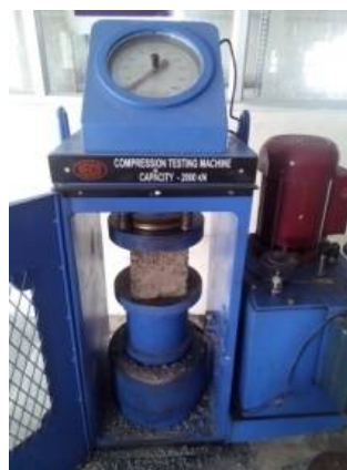
Fig 4.1 Test Set up for Compressive Strength Test
