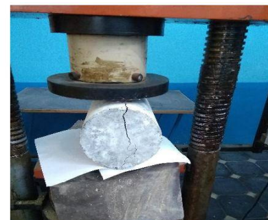
Fig 5 Split tensile strength test
