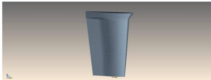
Figure 9. Schilling rudder geometry
