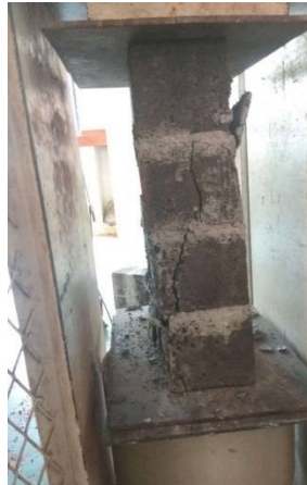
Fig 2: Failure of masonry prism
