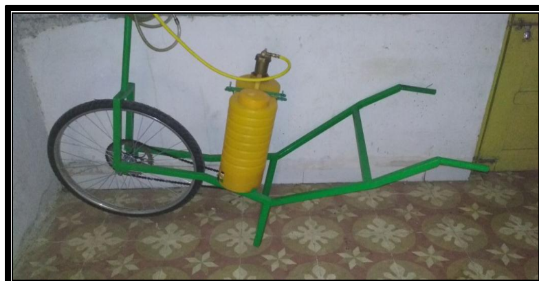
FIG.1 IMAGE OF MANUALLY OPERATED MULTI NOZZLE SPRAYER
