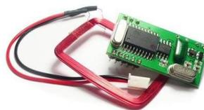
Fig 3: Example of a RFID Reader
