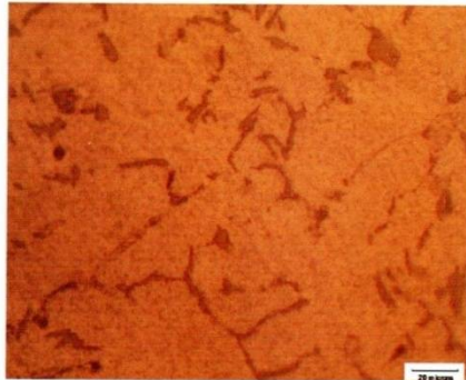
500X keller's Figure 1: Microstructure of A357 As-Cast
