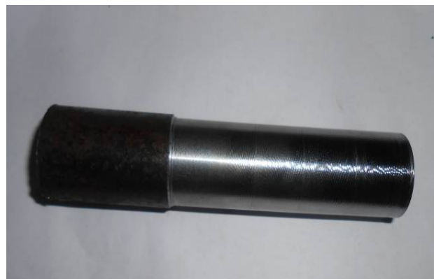
Fig 2: Work piece after turning
