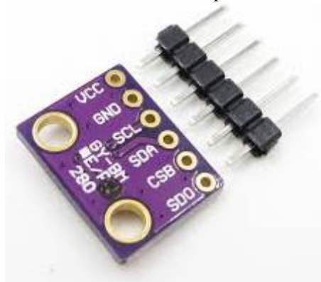
Fig 6- BMP280 - Sensor for determining barometric pressure
