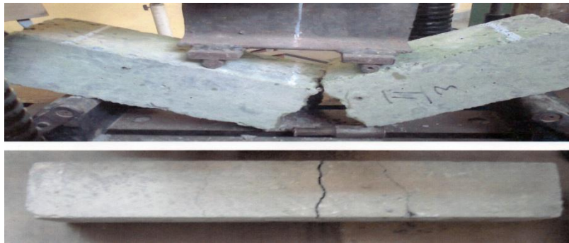
Fig 7: Flexural strength test on beam
