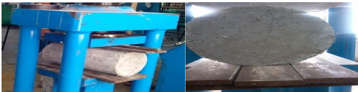
Fig6: Split tensile test of cylinder
