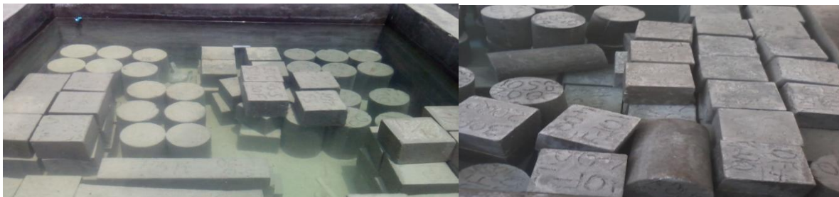
Fig4: Curing tank above figure shows a curing tank in which concrete is kept for 3, 7, 28, 56, 90 days for hydrating of concrete.
