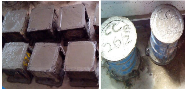
Fig 3: Sampling of concrete above figure shows casting of concrete cubes, cylinders and prisms.
