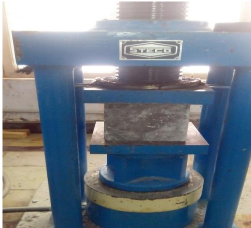
Fig. 3. Testing of cube in compression testing machine
