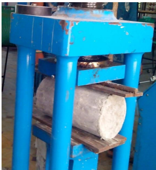
Fig. 4. Split tensile test of cylinder
