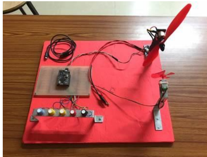
Fig. 4 Hardware of PID and FOPID Control System for PMDC Generator
