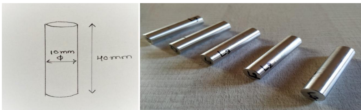
Fig: 5 Dimension of wear test specimen
