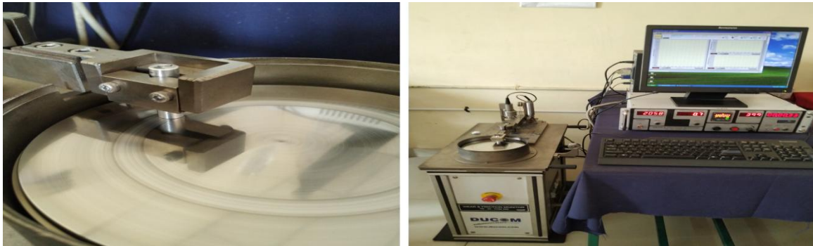
Fig: 6 Wear Testing Setup
