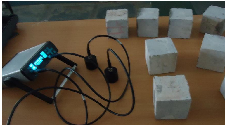
Fig. 2: UPV test Apparatus and concrete specimens
