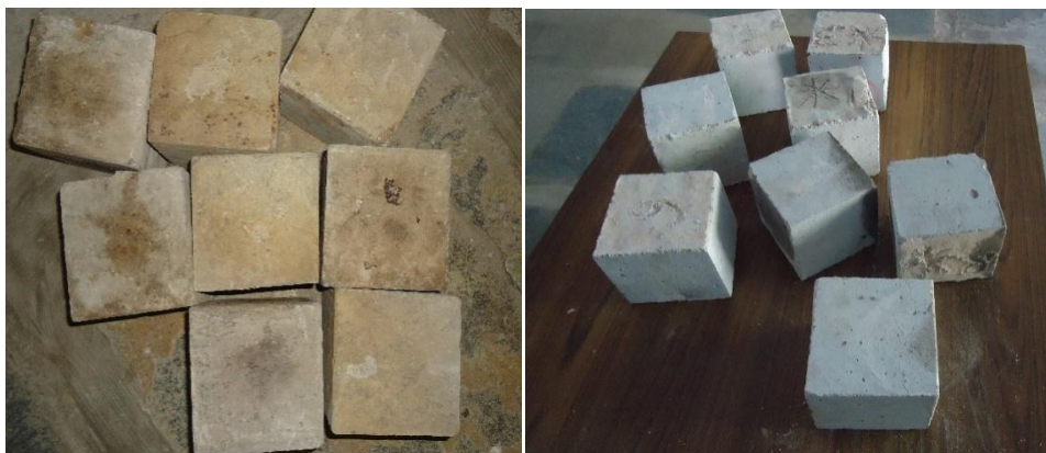
Fig. 4: Cube specimens after subjected to 400 °C and 800 °C
