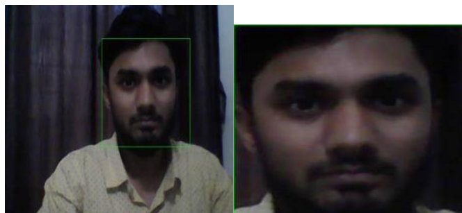
Fig. 2 Face detection result (a) face detection with bounded box and (b) face cropped region
