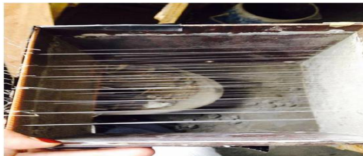
Fig 2 Inserting of optical fibers
