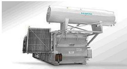
Large oil-filled power transformers will have radiators to cool the insulating oil (left side of this photo); some units rely on natural circulation of oil through the radiator, others use pumps. Often transformer radiators will have fans to increase air flow and transformer power rating. Radiators are found in fluid power systems and air compressors to cool working fluids.
