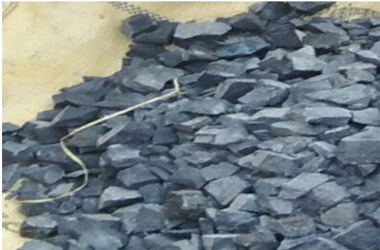
Fig: 1 Shabath rock waste source manual cutting and preparation of aggregates
