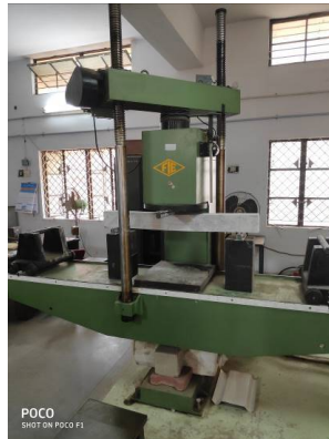
Fig. 3.4 Creating Fault Plane Using Leaf Spring
