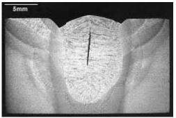
Cracking occurs in aluminium alloys because of high stresses generated across the weld due to the high thermal expansion (twice that of steel) and the substantial contraction on solidification - typically 5 % more than in equivalent steel welds.
