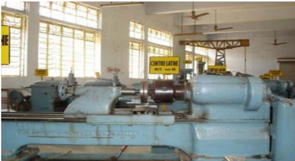
Fig-3 Experimental set-up for Friction Welding
