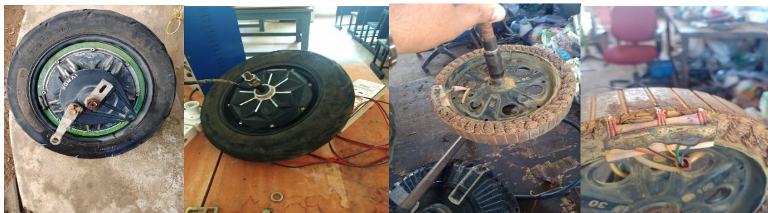
Fig 11: Rotor Or Wheel, Stator and Hall Sensor part of Romai 60 V , 1000W Hub Motor
