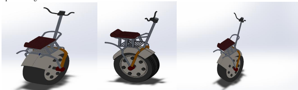
Fig 10: Solid Works 3D Modelling of Uni-wheel Bike
