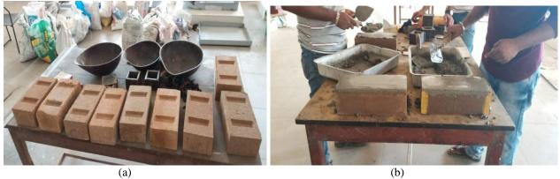
Figure(a) blocks kept for dry testing, figure (b) blocks tested as per IS 3495 (part1) 1992
