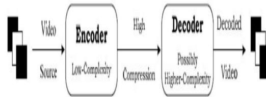
**Figure 1: Ideal coding architecture for upcoming video applications**
