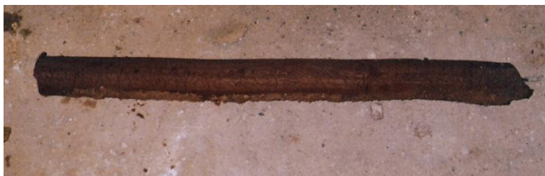
Fig 3.0 Fly ash- Red clay stemming material
