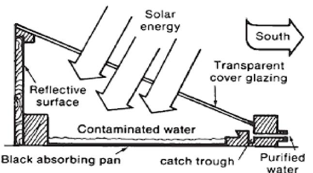
Murasehave analyzed a specific problem associated with the feeding system of a roof type solarstill and they have also analyzed a specific problem Associated with the metallic materials i.e. metallic materials would not be suitable for the construction of solar stills with low productivity. Copper Nickel alloys have been widely used for the tube material
