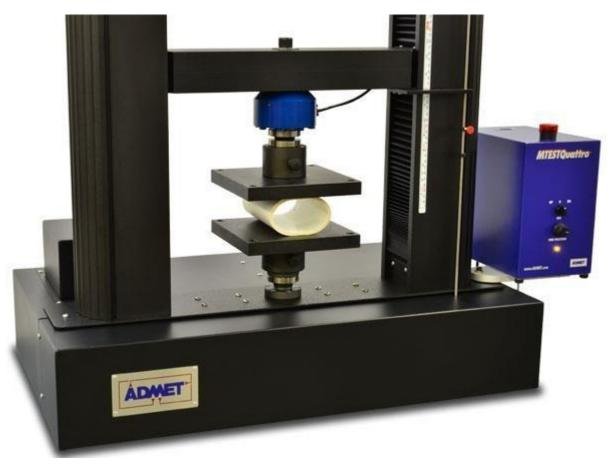
The one of the testing method which is used to establish the behavior of metallic materials that are subjected to a uniaxial compression stress distributed uniformly over the cross section is called as compression test. The goal of a compression test is to determine the behavior or response of material while it experience a compression load by measuring fundamental variable such a asstrain, stress and deformation.
