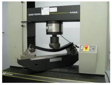
The maximum stress at the outcome fiber on either the compressionon tensile side of the specimen. This
