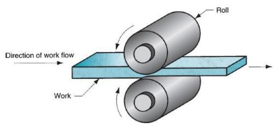
Rolling is the process of reducing the thickness or changing the cross section of a long work piece by compressive forces applied through a set of rolls, as shown in figure.
