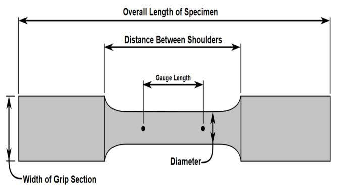
Tensile testing also known as tension testing is a fundamental materials science and engineering test in which is subjected to a controller tension until failure. It's a destructive test process that provides information about the tensile strength yield strength and ductility of the metallic material.
