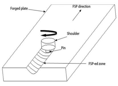
Stir processing expands the improvement of FSW (friction stir welding).FSW is build up in welding institute of the United Kingdom in 1991. FSP is a new thermo mechanical technique to achieve good performance with less production cost in a min. Time and it's also achieve better microstructure & mechanical properties in a single pass.
