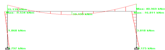
Fig 11 Bending Moment (ASCE 7-10)
