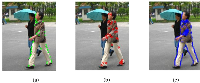
Fig. 1. Features detected in the first scenario by a) Harris detector, b) Harris-Laplacian detector and c) Laplacian of Gaussians detector. Source: Own elaboration.
