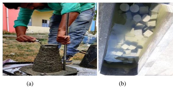
Fig.4.2.(a)(b).slump cone test &Curing Tank
