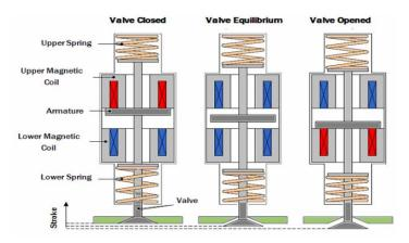
Figure 2. Simplified working diagram of an EMV actuator
