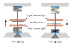
Figure 1. Valve actuation while closing and opening of valve
