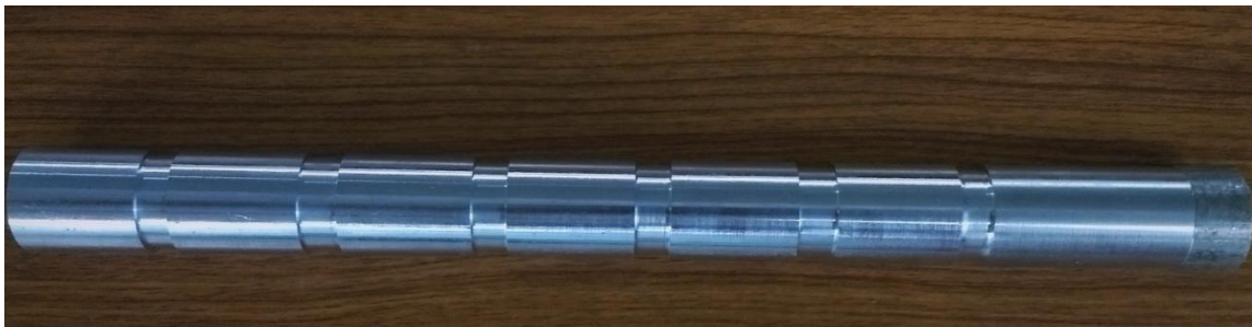
Aluminium specimen after turning and grooving
