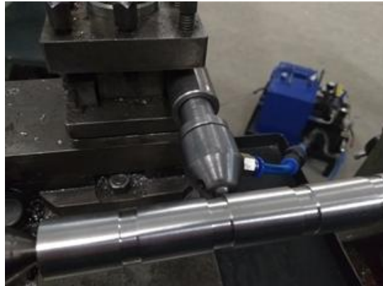
Burnishing process carried out on the specimen
