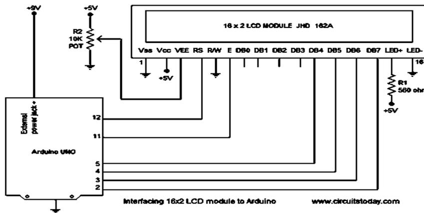
Fig 2: Interfacing Diagram
