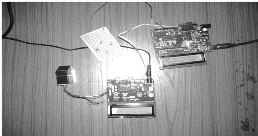
Fig 7: Circuit for Biometric authentication
