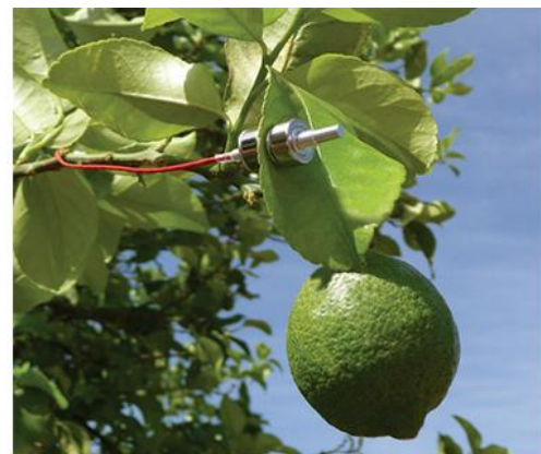
Water potential sensor installed on lemon tree
