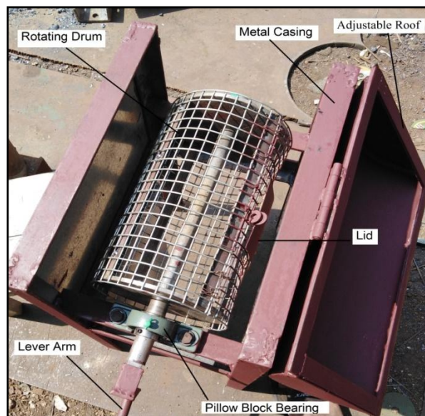
Fig.5. Fabricated Hot air dryer
