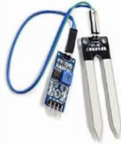
Fig 3. soil moisturing sensor
