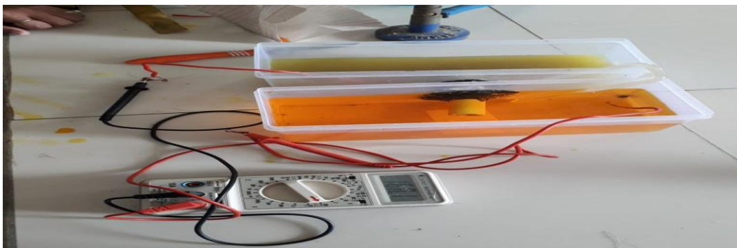
Fig 2: Design set up of Salt Bridge
