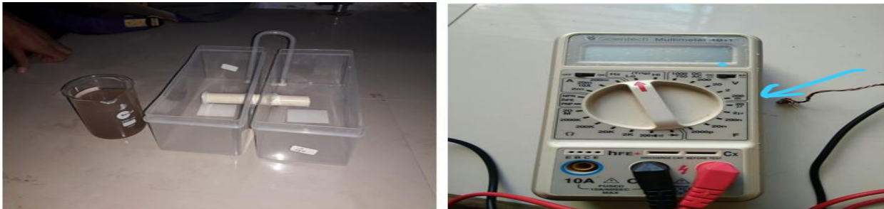
Fig 1: Salt Bridge Construction for treating wastewater and Multimeter for measuring current.
