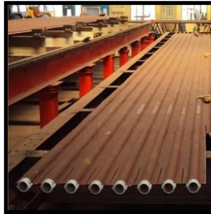
Fig: 1.3 Boiler Panels
