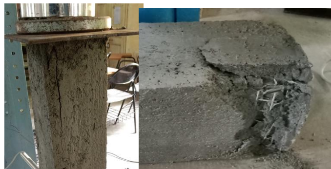
Fig-9 Crack and failure pattern of retrofitted specimen
