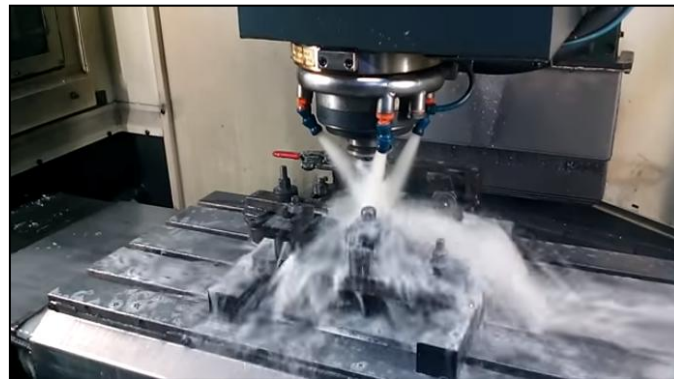
Fig. 5 Taguchi Specimen For MQL
