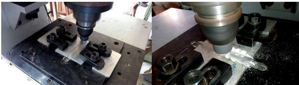
Figure 1: (a) FSW Process using conventional milling machine.
