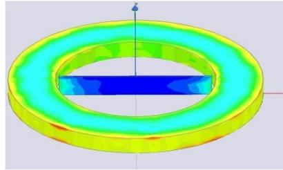
Flux density magnitude diagram of ring magnet
