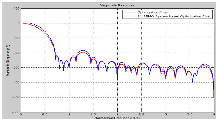
Figure 5: MagnitudeResponse of  $2 \times 1$  MIMO system based Optimization Filter
