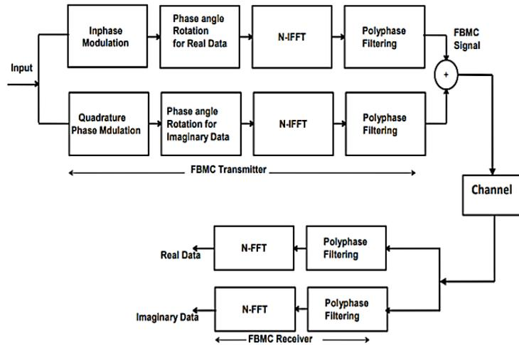
Figure 2: Block diagram of FBMC transceiver
