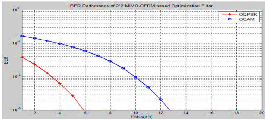
Figure 9: BER Analysis of 2x2MIMO system based Optimization Filter
