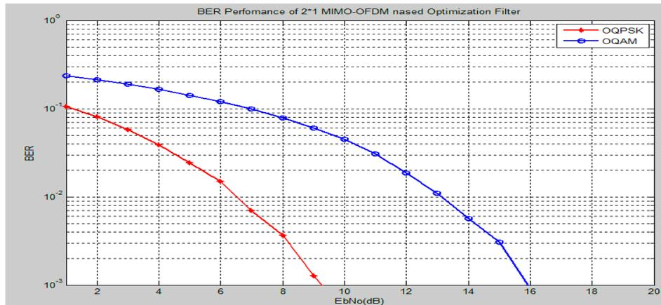
Figure 6: BER Analysis of 2x1 MIMO system based Optimization Filter
