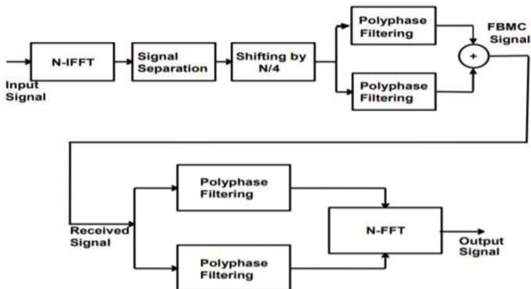
Figure 3: Simplified FBMC transceiver
