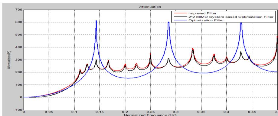
Figure 7: Attenuation Graph of 2x2 MIMO system based Optimization Filter
