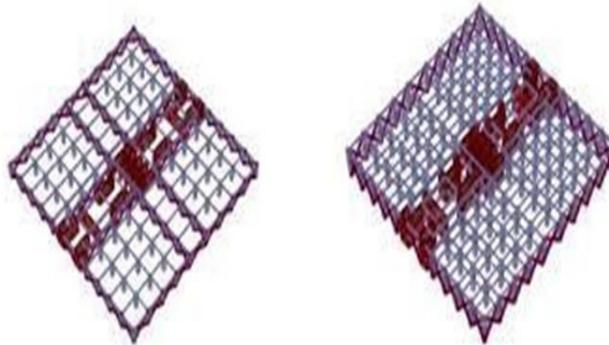
Fig 1.3 Conventional outrigger system and Virtual outrigger system
