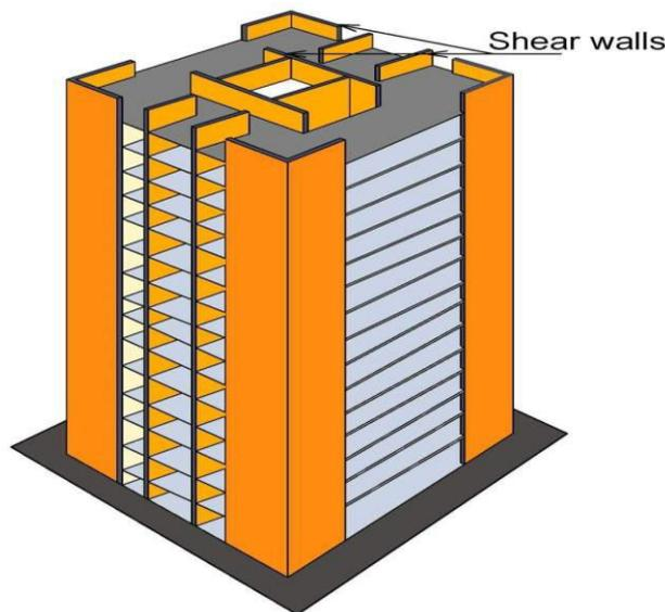
Fig 1.5 Building with Shear wall
