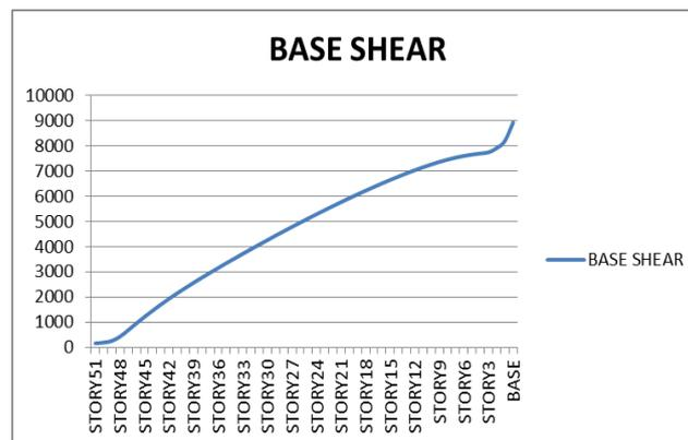
Graph 5.3 Base shear with shear wall
