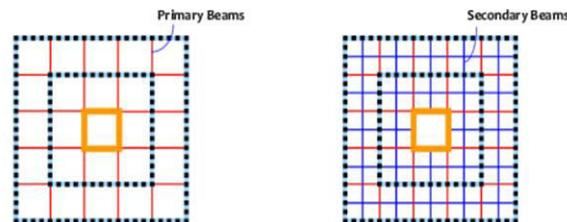
**Fig 1.2** Beams in Tube-in-Tube Systems: Secondary beams help in transferring the gravity loads to the two tubes and the core.
